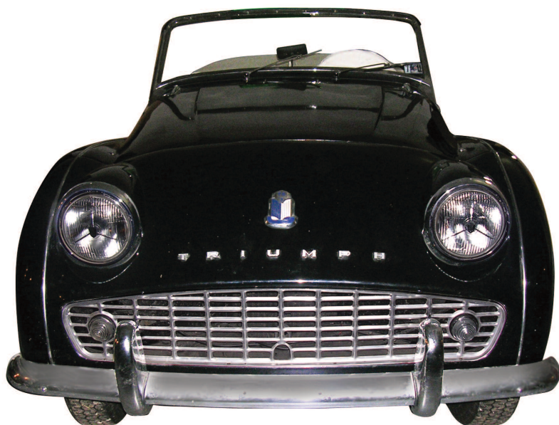
TR3A Fitted with Original Lucas PL700 Tripod Headlamps and the 802174 Grille
