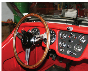
PHOTO LEFT SHOWS A MOTO-LITA WOOD-RIMMED STEERING WHEEL AND TRF'S SIGNAL SWITCH/HORN PUSH (CONTROL HEAD) FITTED TO JOHN SWAUGER'S 1958 TR3A.
