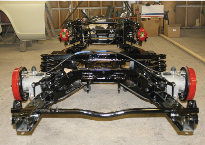
Rear View of Chassis Ready for Installation of Differential
