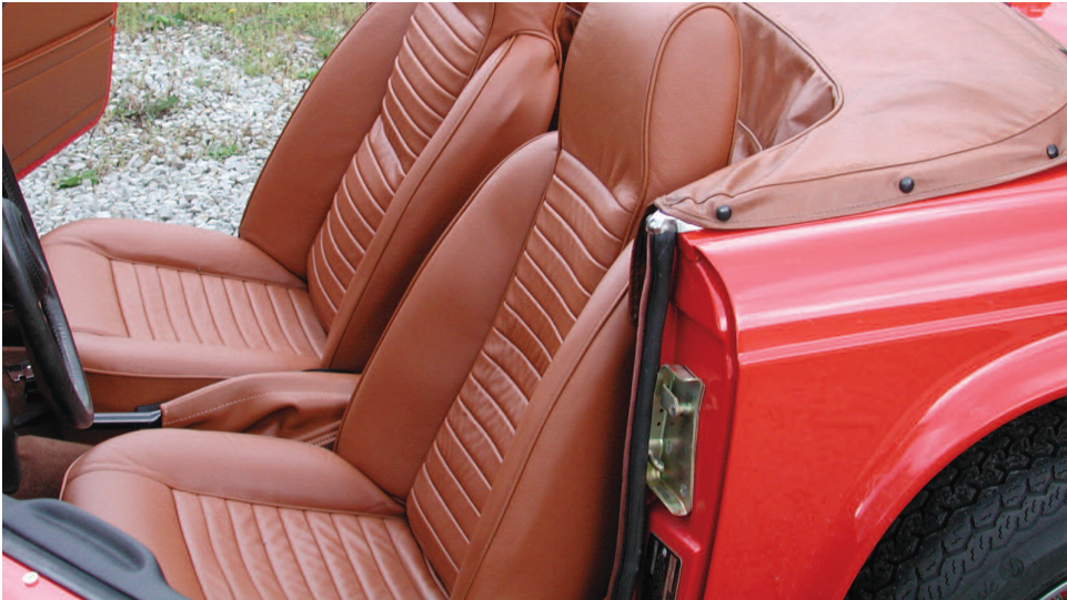
TR6, Showing Rear Door Post with Dovetail Fitted
