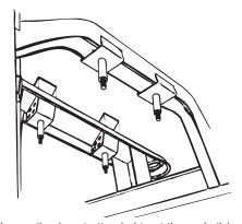
If the problem of a cracked mounting is not attended to at the early "clunk" stage, then additional stress will be placed upon the chassis frame at the point where the upper end of the bolt is welded to the rear suspension crossmember. Sooner rather than later, stress cracks will appear at this point, adding to the expense of the repair and increasing the risk of additional problems and failure on the road.
